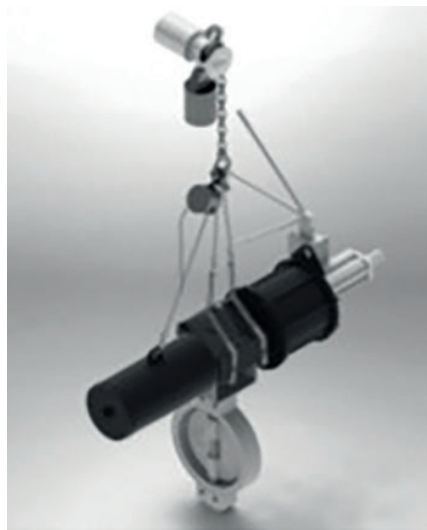
Figure 4-2: Sample lifting points for valves
