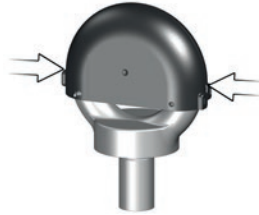
Fig. 4-3: Eyebolt cover in place on the eyebolt
