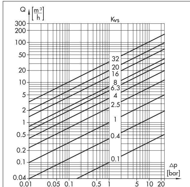
Terms for control valve sizing for other media according to IEC 60534 Part 2-1:  $F_L = 0.95$  and  $x_T = 0.75$
